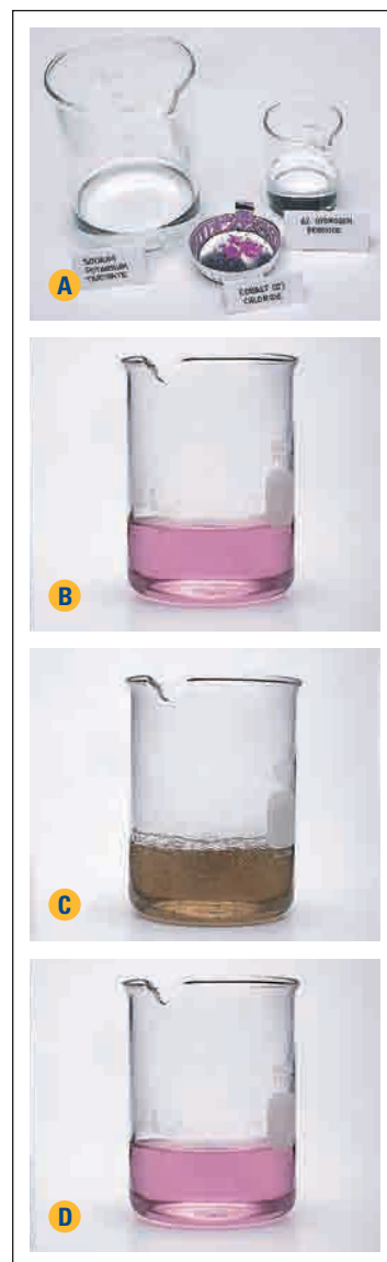
Figure 6.19 The reaction of Rochelle's salt, sodium potassium tartrate, with hydrogen peroxide is catalyzed with \text{CoCl}_2 at 70^\circ\text{C} .
