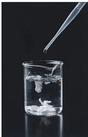
Figure 9.7 A chemist can test for the presence of chloride ions in a solution by adding silver nitrate solution. If a white precipitate of silver chloride forms, the test is positive for chloride.
