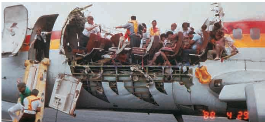
Figure 11.27 On April 28, 1988, this Aloha Airlines aircraft was flying at an altitude of 7300 m when a large part of the upper fuselage ripped off. This accident was caused by undetected corrosion damage. The pilot showed tremendous skill in landing the plane.
