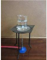
The following image shows the correct setup for heating liquids on a Bunsen burner:
